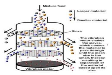
Fig no:1 Screening method of size separation
