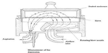
Fig no 9: diagrammatic representation of alpine air jet sieves
